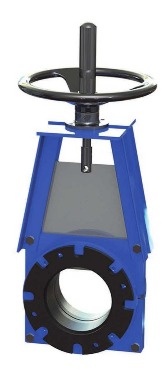
The Flanged Slurry Knife Gate Valve KGA - FGV is built with a cast SG Iron GR. 42 or fabricated body and features a heavy-duty stainless steel blade. Removable seats on either side of the blade provides a bi-directional, bubble-tight seal with no metal parts in contact with the slurry.
