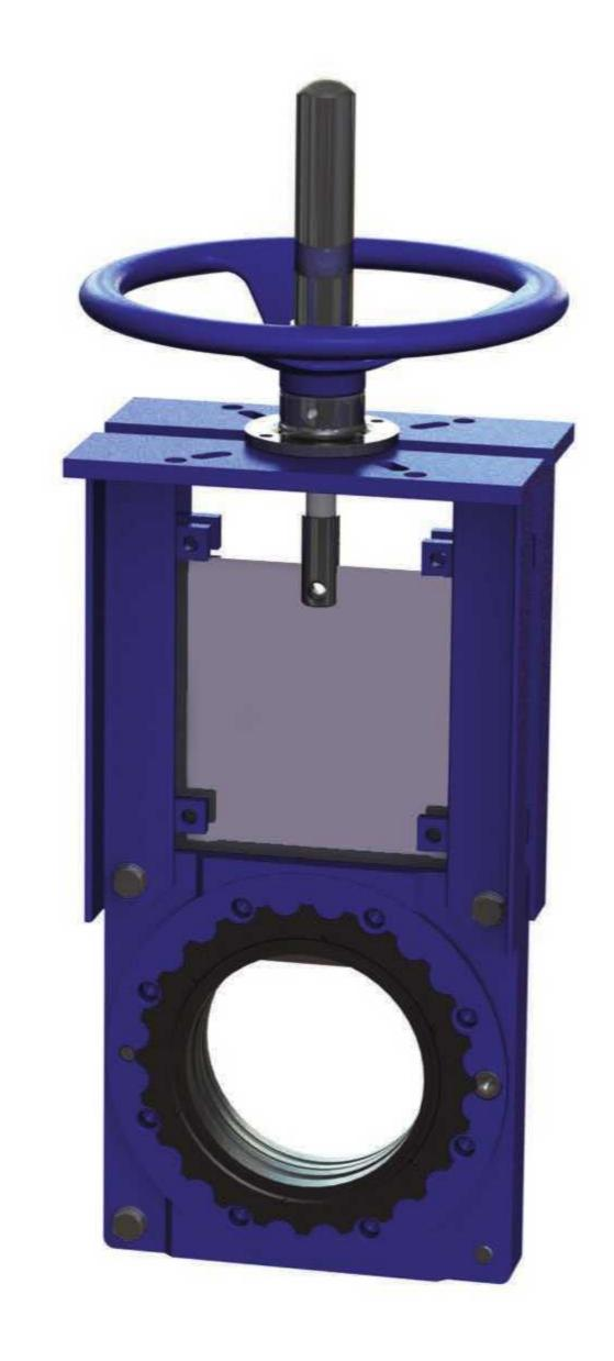
The Slurry Wafer Knife Gate Valve KGD - WGV, is built with a cast body and features a heavy-duty stainless steel blade. Removable seats on either side of the blade provides a bi-directional, bubble-tight seal with no metal parts in contact with the slurry.
